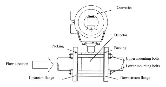
Figure 4.4 LF516/LF546 flowmeter piping connections
